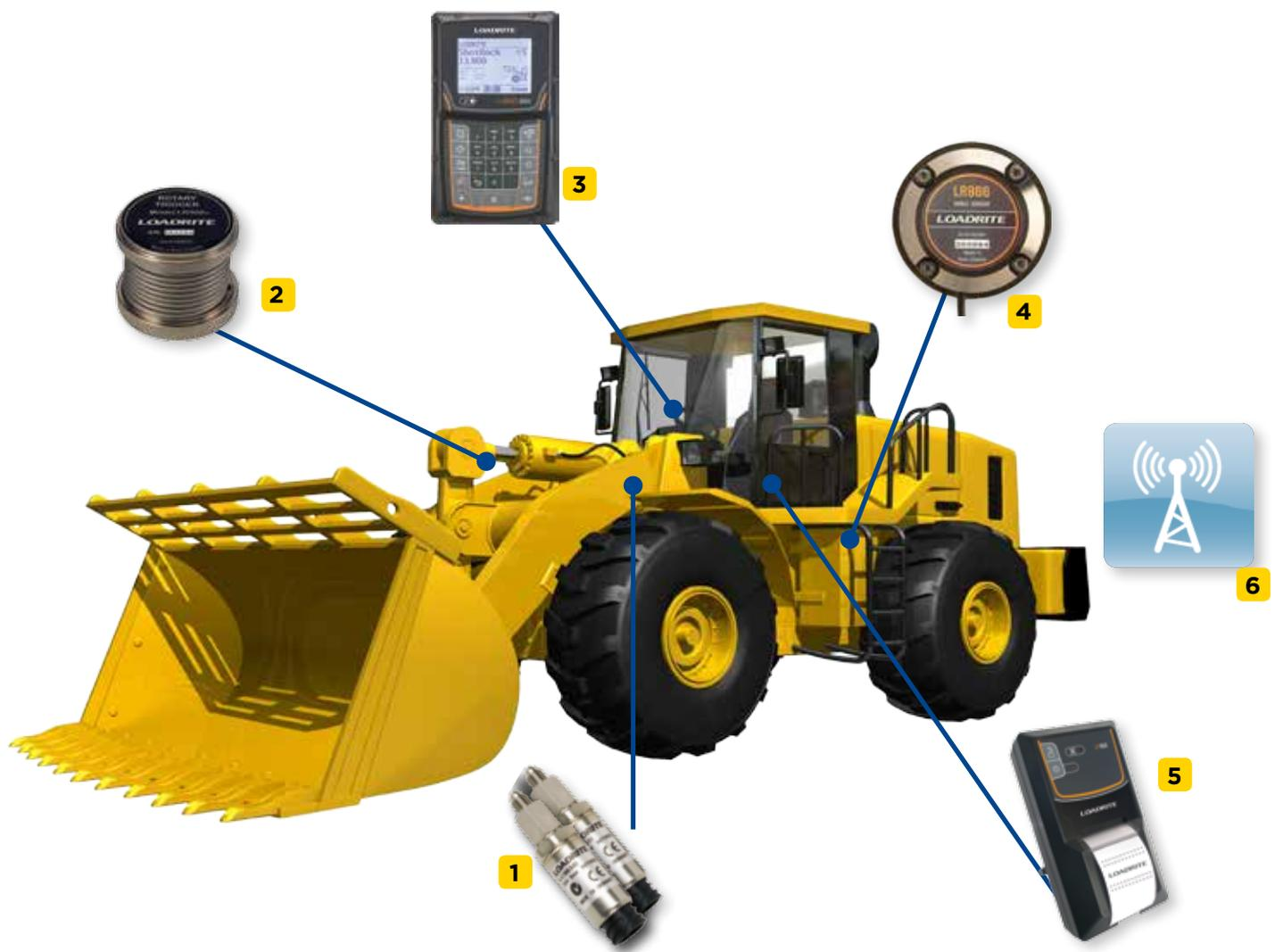
**Pressure Transducers:** The pressure transducers connect to the loader's hydraulic system. They sense the hydraulic pressure in the lift cylinders as the load is lifted.
