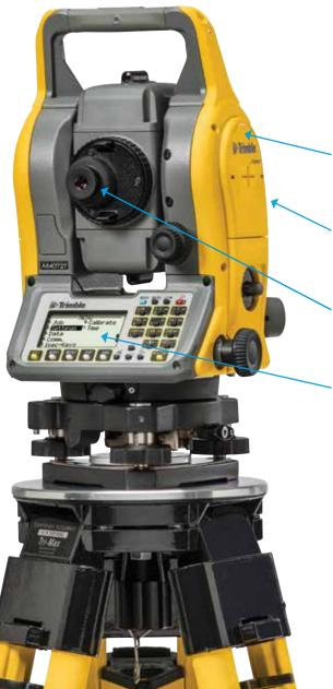
Dual lithium-ion batteries for up to 19 hours of continuous use
